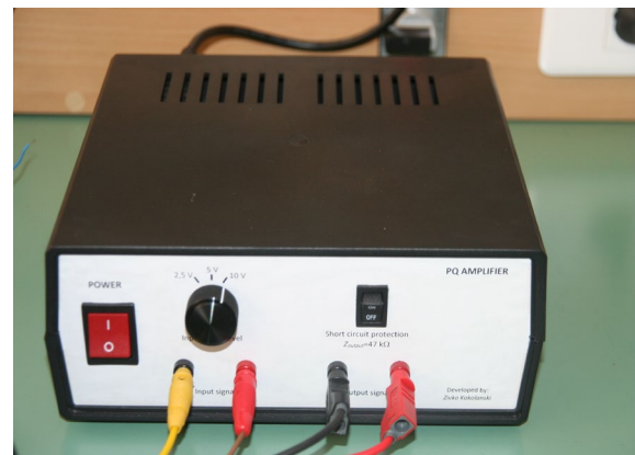
Fig. 9. Practical realization of the PQ amplifier
